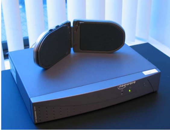
Figure 4: The Ethernet Speaker is based on the Neoware EON 4000.
